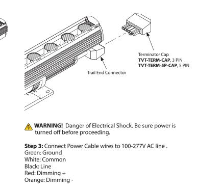
**Step 2:** Insert Terminator Cap into the female Trail End Connector.
